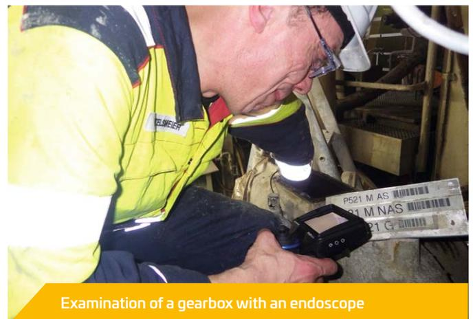
Examination of a gearbox with an endoscope
