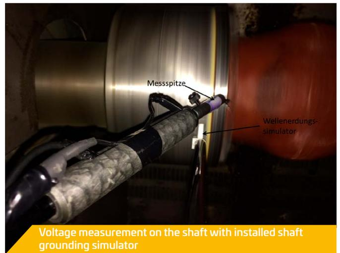
Voltage measurement on the shaft with installed shaft grounding simulator
